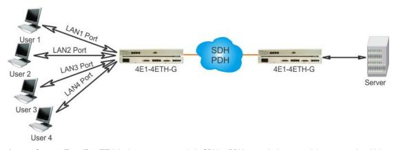
**Access Server** - Two 4E1-4ETH devices are connected via SDH or PDH transmission network interconnection. Using GFP and VC technology get together 1~4E1 and provide 4×2Mbps transmission channel bandwidth used to transport Ethernet services. Transmission channel bandwidth dynamic adjustment using LCAS technology.
