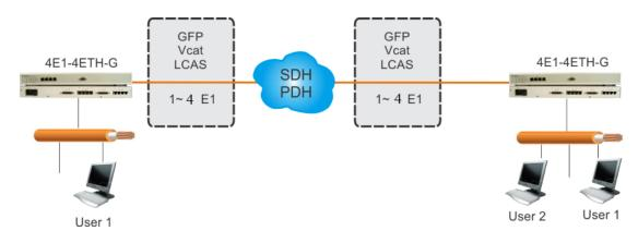
**Device networking application** - unit's are connected to using 4E1 lines directly to PDH or SDH network, and special interconnection features are possible at SDH level due to GFP-F, VC and LCAS technology support.
