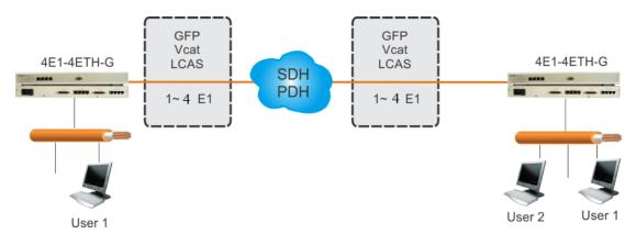
**Device networking application** - unit's are connected to using 4E1 lines directly to PDH or SDH network, and special interconnection features are possible at SDH level due to GFP-F, VC and LCAS technology support.
