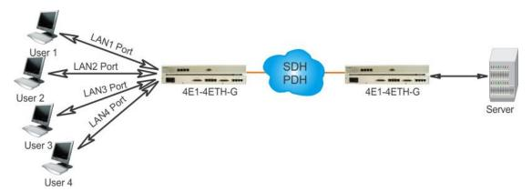
Access Server - Two 4E1-4ETH devices are connected via SDH or PDH transmission network interconnection. Using GFP and VC technology get together 1~4E1 and provide 4×2Mbps transmission channel bandwidth used to transport Ethernet services. Transmission channel bandwidth dynamic adjustment using LCAS technology.
