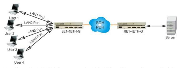
Access Server - Two 8E1-4ETH devices are connected via SDH or PDH transmission network interconnection. Using GFP and VC technology get together 1~8E1 and provide 8×2Mbps transmission channel bandwidth used to transport Ethernet services. Transmission channel bandwidth dynamic adjustment using LCAS technology.
