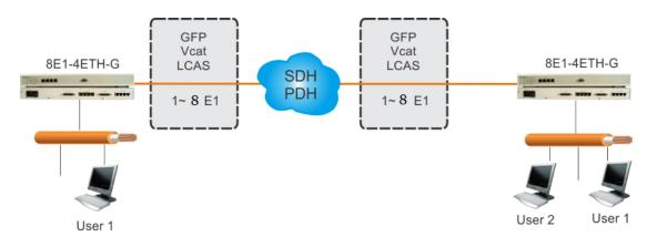
**Device networking application** - unit's are connected to using 8E1 lines directly to PDH or SDH network, and special interconnection features are possible at SDH level due to GFP-F, VC and LCAS technology support.
