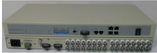
OPTIMUX can provide up to 16 E1 interfaces and 3 fast Ethernet + 10/100M optical Ethernet port. The Ethernet interface can be operated in 10M/100M, half duplex or full duplex mode by either auto-negotiation or manual setting.
