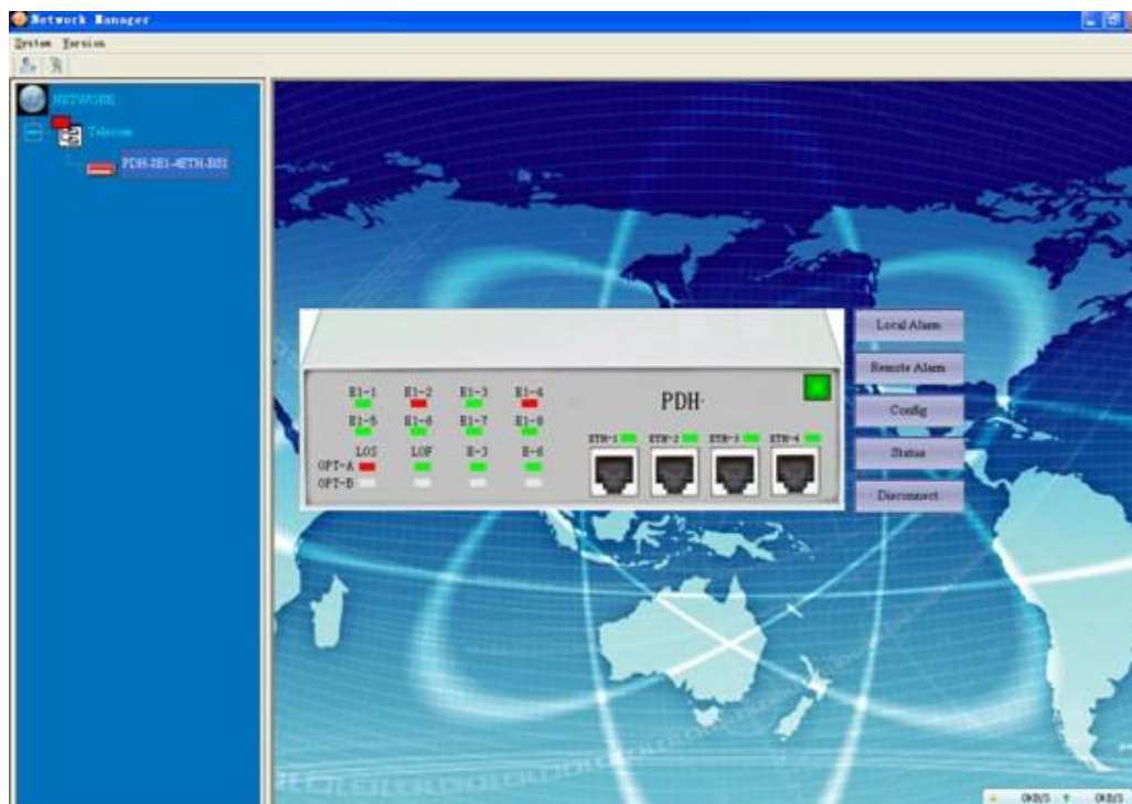
Alarm history and current alarms via RS232 GUI NMS
