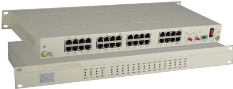
This product is elementary equipment for digital communication system, also called PCM group bank equipment. It gathers signals such as FXS FXO, Ethernet, RS232/422/485, V.35, E&M... into a standard 2M E1 interface and achieves the point-to-point transmission of these signals .
