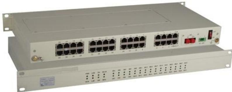
This product is elementary equipment for digital communication system, also called PCM group bank equipment. It gathers signals such as FXS FXO, Ethernet, RS232/422/485, V.35, E&M... into a optical interface and achieves the point-to-point transmission of these signals
