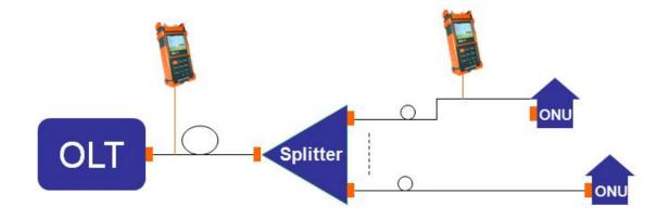
In-service testing (1625nm with filter)
