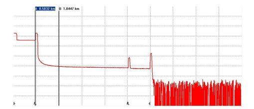
Testing through ≥1x64 splitter, splitter and fiber end identifiable
