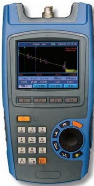
The **WY-8100 OTDR** is a high performance mini-OTDR, which is small in size, light in weight and rugged in configuration. Very suitable for measuring unit、connection、transmission loss and locating faults or breaks on optical fibers.
